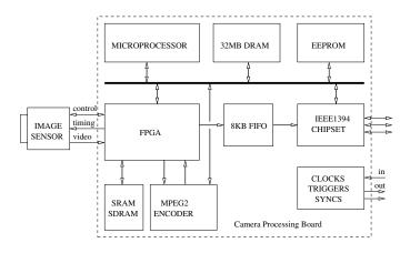
Figure 3: Camera processing board block diagram
